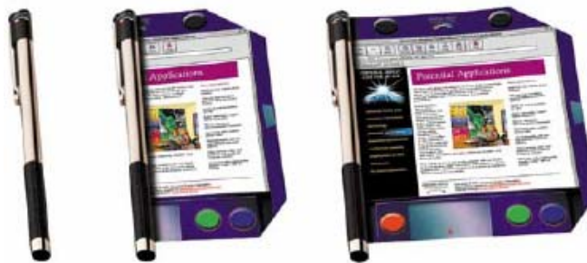
Figure 10. A prototype model of a potential flexible flat panel display application. The device could be rolled up into a pen when not in use. Images courtesy Universal Display Corp, from ref. 25.
