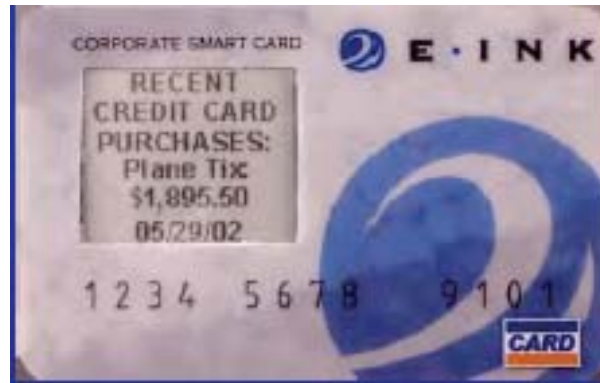
Figure 9. Photograph of “smart card” application. The display is created using E-ink® electrophoretic technology ( www.e-ink.com ).
