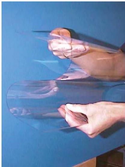
**Figure 4. Photograph showing thin, flexible glass.<sup>26</sup>**
