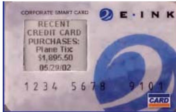
Figure 9. Photograph of “smart card” application. The display is created using E-ink® electrophoretic technology ([www.e-ink.com](http://www.e-ink.com)).
